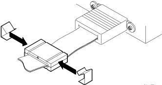
When properly installed, the ferrite should appear on the logic analyzer cable as shown.
